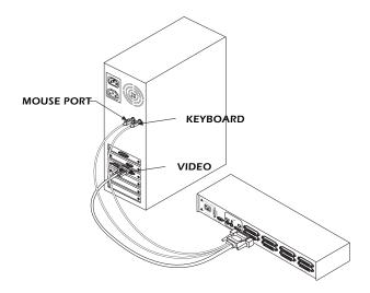
3. Locate your next input cable. Repeat step 2 with all the computers that will be attached to your master switch. Next, attach the remaining computers to the slave switch.
